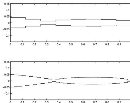
Figure 3: Discretization of the beam with endpoints fixed-simply supported by using 8 ( $J=29.458$ ) and 32 elements ( $J=15.765$ ) respectively.
