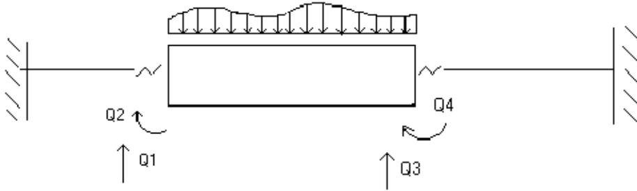
Figure 1: Generalized forces at one element of the beam.
